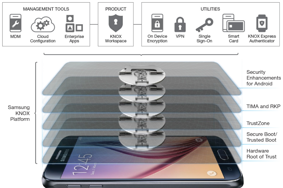
Figure 1 – Samsung Knox Platform, Workspace, Management Tools and Utilities
