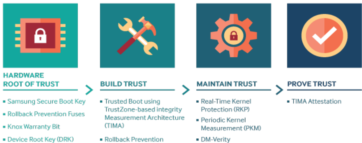
Figure 2 - Knox Builds, Maintains and Attests Its Trusted Environment
