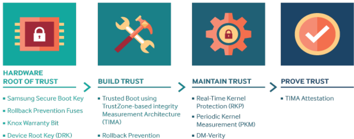
Figure 2 - Knox Builds, Maintains and Attests Its Trusted Environment
